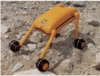
Gofor, with active center of gravity compensation. (c)
